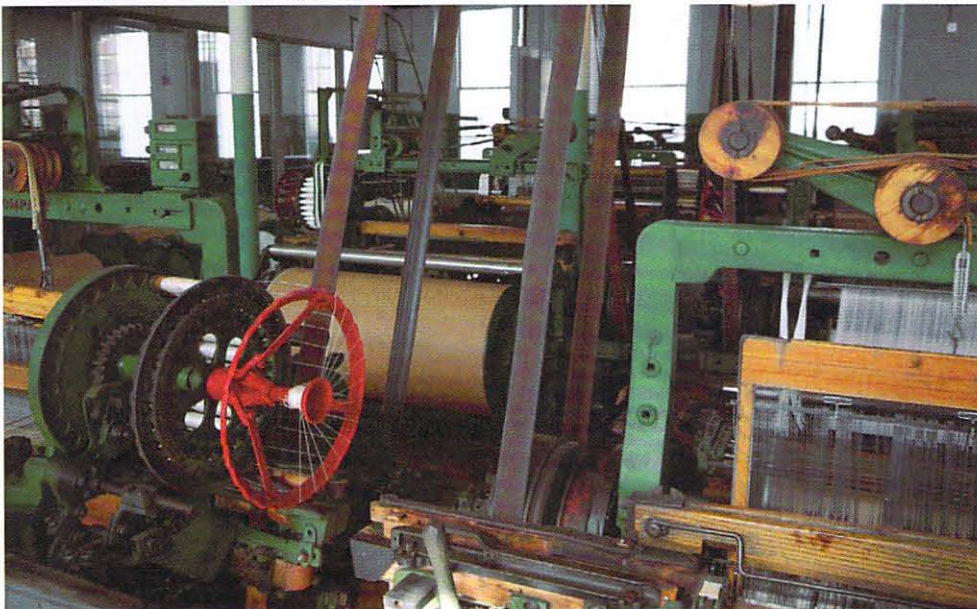
At the start of the Industrial Revolution, factories using specialized machines began to replace hand spinners and weavers in the production of cloth. These historic mechanical looms can still be seen in operation at a museum in Lowell, Massachusetts.
